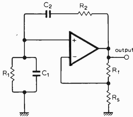
$$f = \frac{1}{2\pi\sqrt{R_1 C_1 R_2 C_2}}$$
