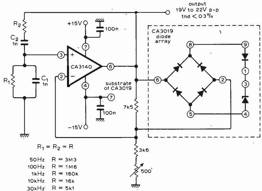
otherwise the amplitude will either diminish or limit. In the full circuit  $R_s$  is formed by a zener diode shunting the feedback resistor  $R_f$ . As output signal amplitude increases, the zener diode impedance decreases and reduces the gain, thus stabilizing the output amplitude.
